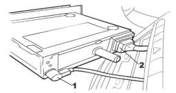
With the main radio cable removed, first connect the Dension supplied cable to the original factory cable harness.
