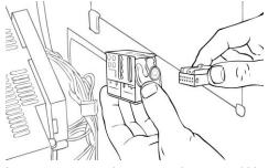
In some cases there may be an add-in connector. Remove the CD changer section and replace with the loom supplied with the Gateway Lite Blue. For further details please go to **section 6**.
